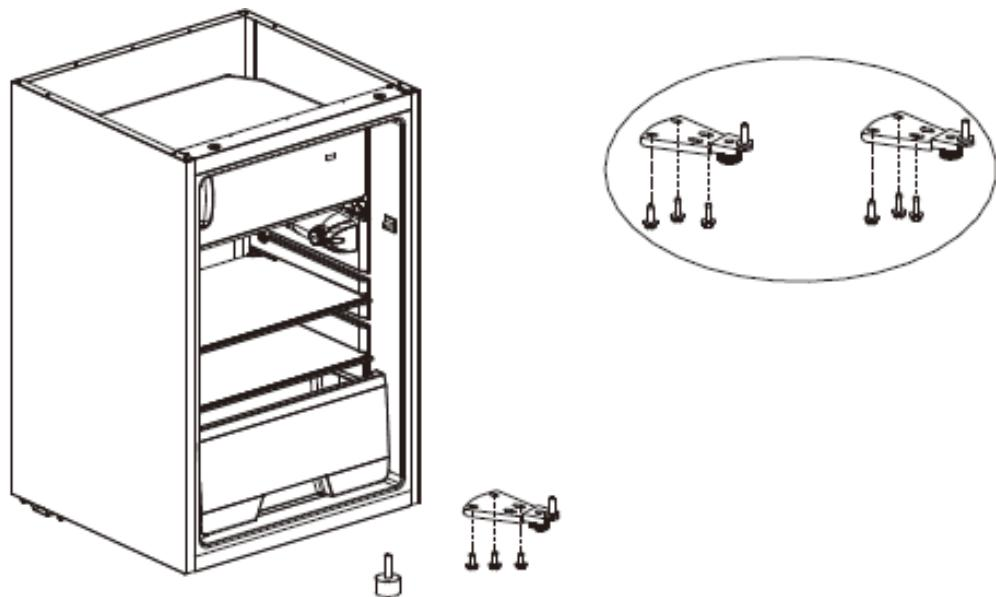
6. Put the door on bottom hinge and assemble the upper hinge, screws, and upper cover.
